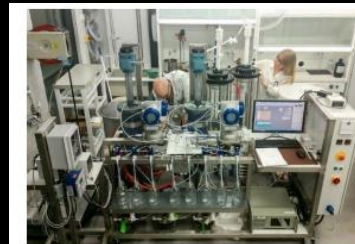
Small scale IX pilot 2 x 12 L bed volume
