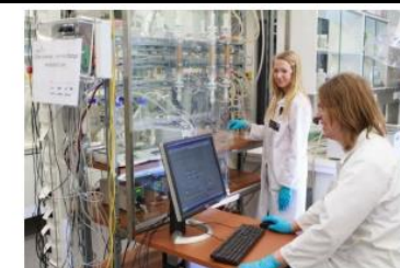
Continuous IX work station 10 x 0.1 L bed volume
