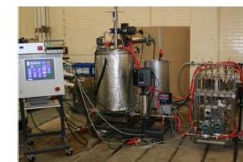
Rotating blade cross-flow filter 1 m 2 filter area
