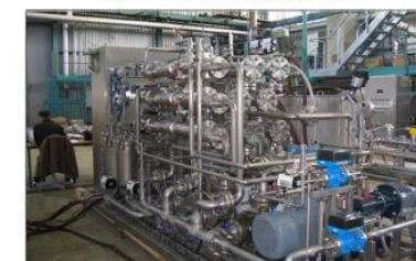
3-stage spiral wound unit 45 m 2 , 5 m 3 /h
