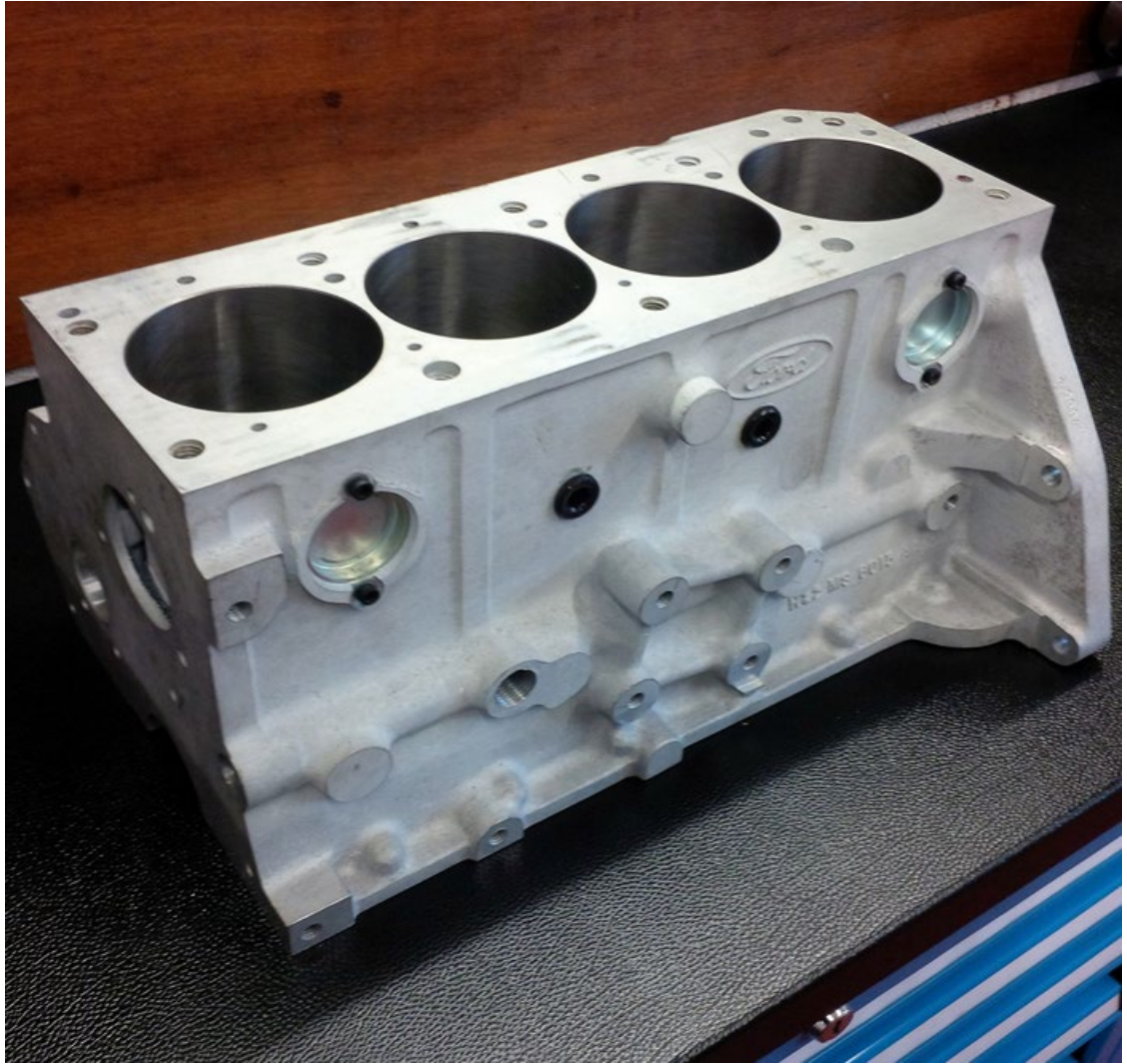
Ford Cosworth BDG cylinder block cast by Grainger & Worrall . The part is modeled after the original, and matches it perfectly. This engine has not been in production by Ford for 35 years. A typical remanufactured part made with 2020 technology.
