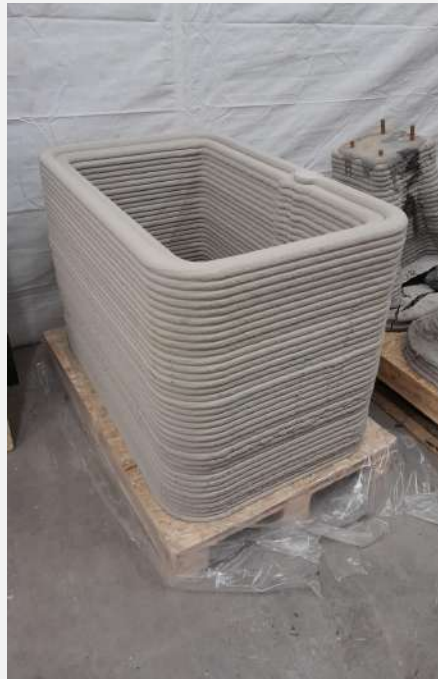
Inspection chambers and manholes
