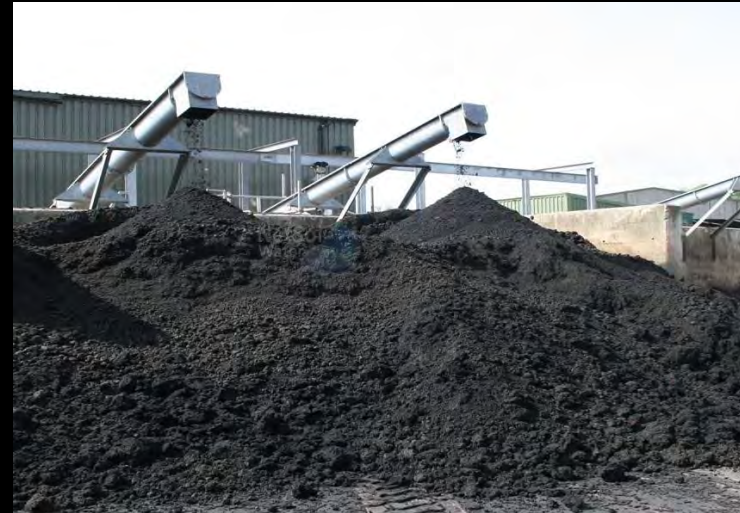
Dewatered sewage sludge
